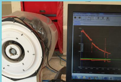
Assemble and install a "Blower Door" to maintain positive pressure in the space.
