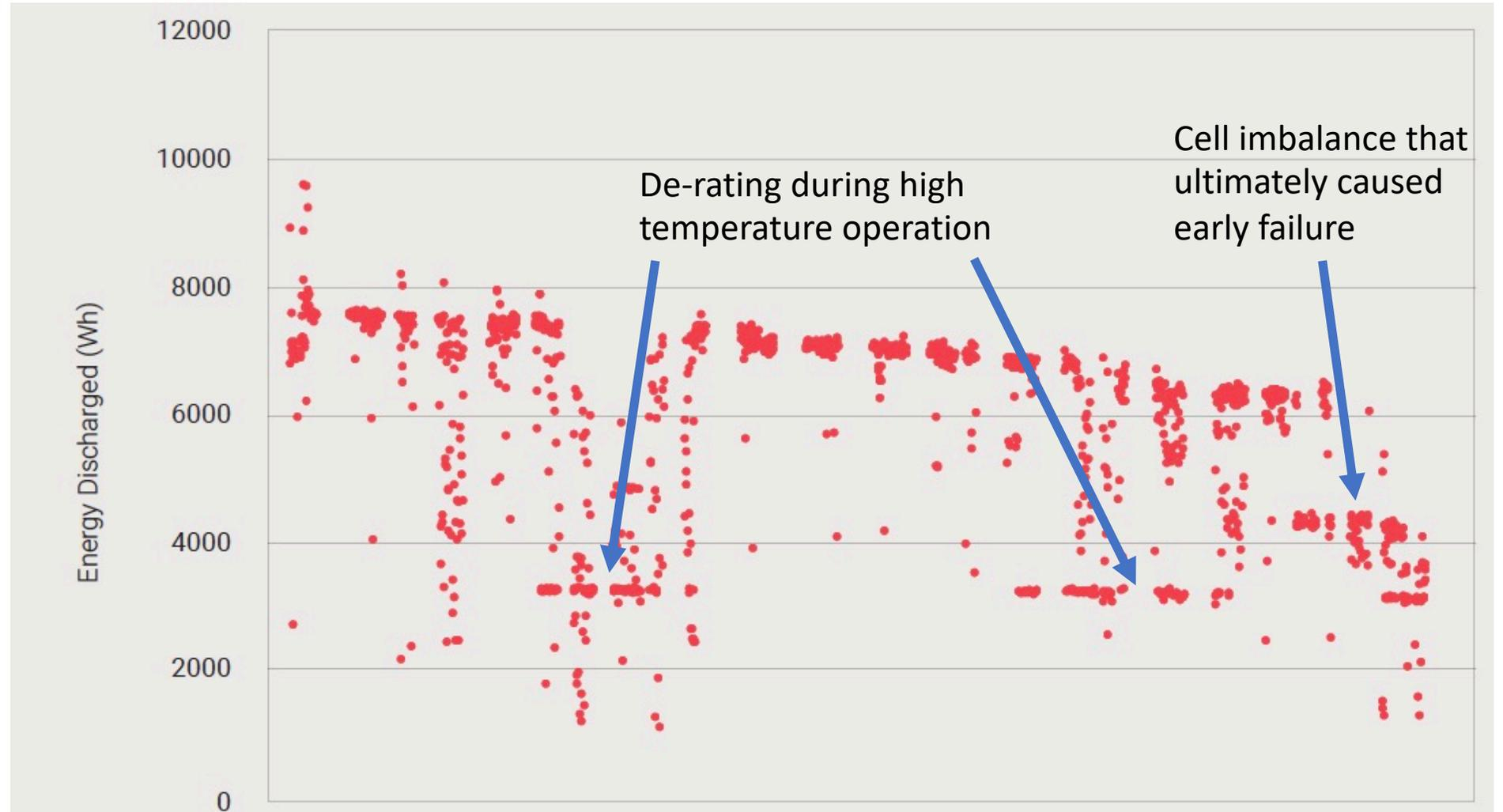
Figure 5. Energy discharged per cycle by the LG Chem RESU 1 battery pack
